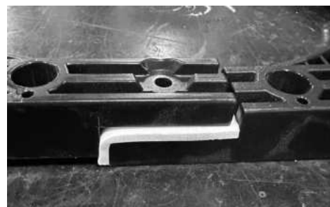
Image 7 Foam Strip Installation
